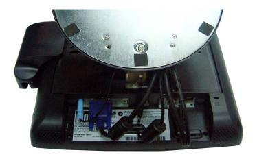
• Connect one end of the MSR cable to the computer and the other end to the monitor.
